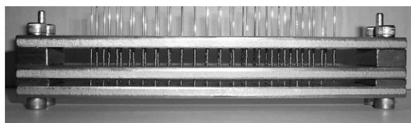
**Fig 3.** Compression rack with GAC International stop-wound coils.
