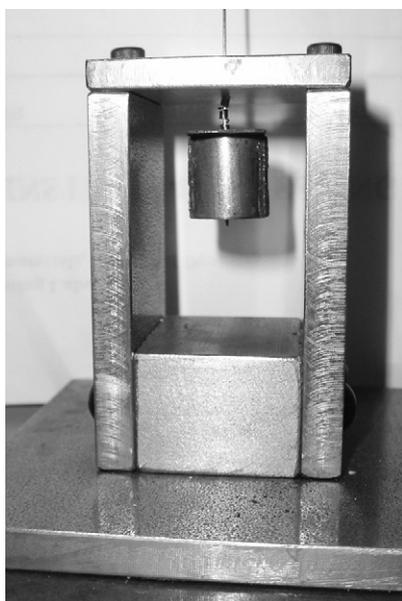
**Fig 2.** Jig attached to the testing machine.
