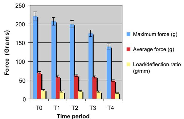
**Fig 4.** Change in force magnitude over time for GAC International stop-wound light springs. The GAC International medium and heavy stop-wound coil springs had similar changes in force magnitude over time.
