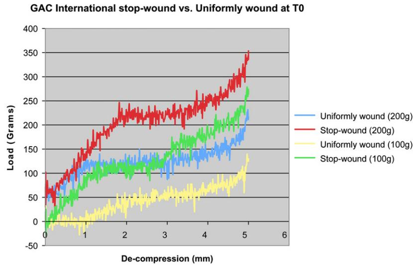
Fig 5. Load-deflection diagram for GAC stop-wound and uniformly wound coils (100 and 200 g).
