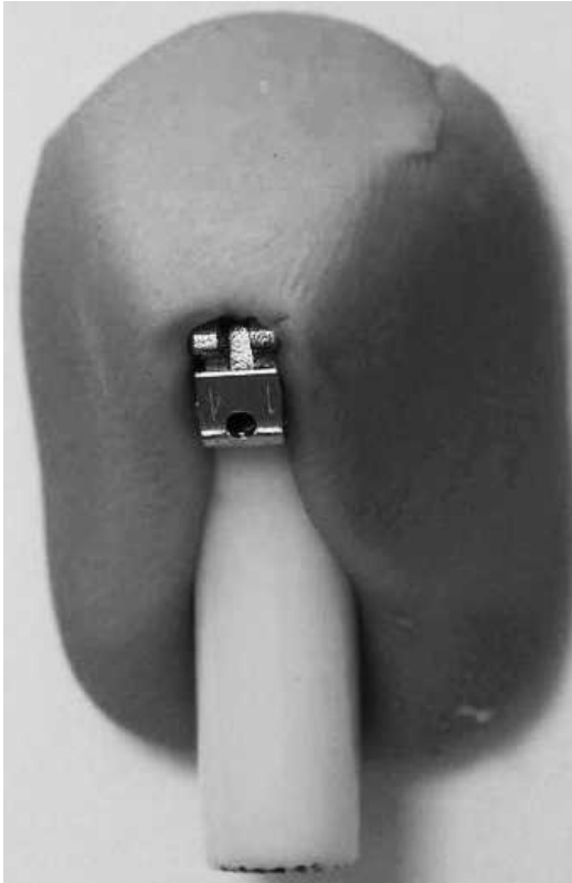
Figure 3. Polyvinyl siloxane bonding jig. Original from Budd et al. 11
